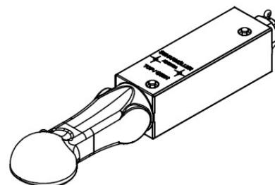
Coupling heads 80 may only be used in conjunction with the type approved, for mounting suitable draw bars, that are suited for coupling ball couplings 80 according to ISO 24347 and that fulfill the required parameters and allow the required horizontal ( $\pm 60^\circ$ ), vertical and axial ( $\pm 20^\circ$ ) pivoting angles.
