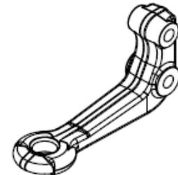
When using the drawbar eye on rigid drawbar trailers it should also be noted that the correlation between the height of the centre of gravity and the effective length of the drawbar (distance between centre of coupling and centre of axle or axle unit) with a permitted total mass of the trailer may not exceed 0,4.
