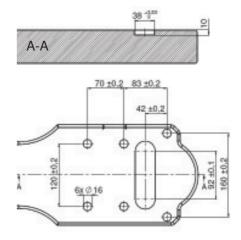
Schraubanschluss / screw connection
