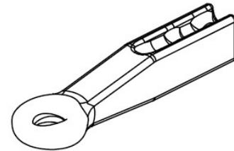
When using the drawbar eye on rigid drawbar trailers it should also be noted that the correlation between the height of the centre of gravity and the effective length of the drawbar (distance between centre of coupling and centre of axle or axle unit) with a permitted total mass of the trailer may not exceed 0,4.
